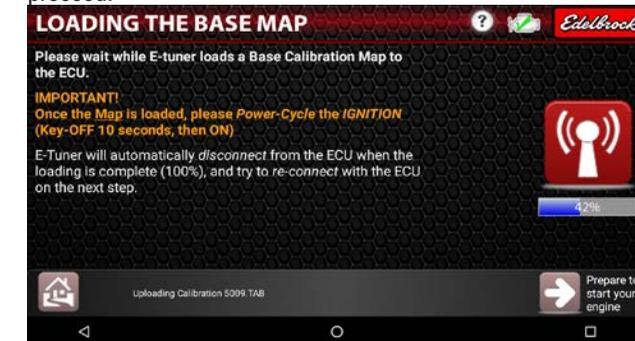
16. Read the important warning then press the Check Mark to continue. **Do NOT start the engine or drive the vehicle until prompted to do so.**
