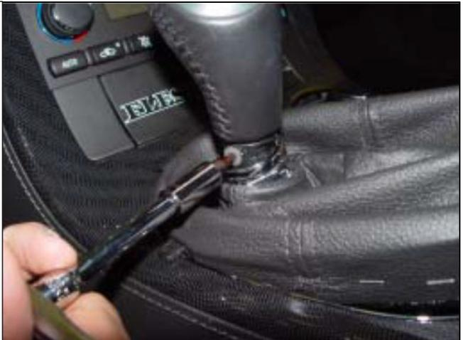
8. Remove center console trim plate from center console. Be sure to unclip any connectors that would prevent the removal of the center console trim plate.
