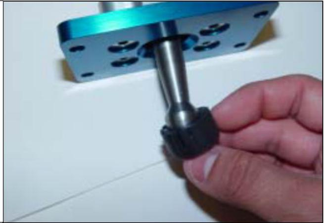
14. Remove the old rubber gasket completely and install the provided gasket.
