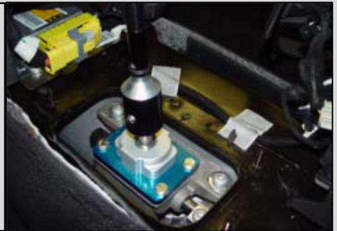
16. Reinstall the second rubber layer, securing the rubber using (4) nuts. Reinstall the first rubber layer.
