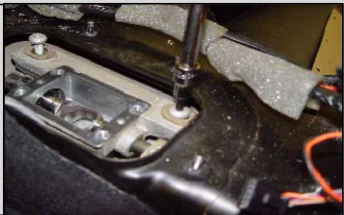
C. Remove the stock rubber bushings and spacer.
