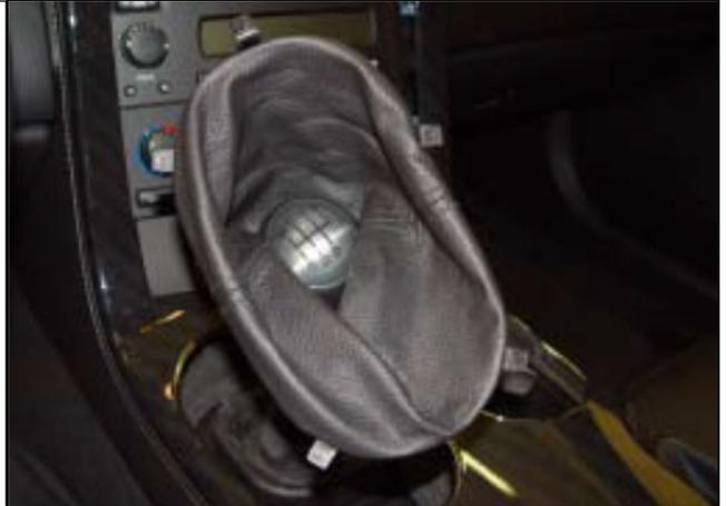
7. Hold top of knob and turn chrome collar counter-clockwise to loosen collar and access bolt securing knob.
