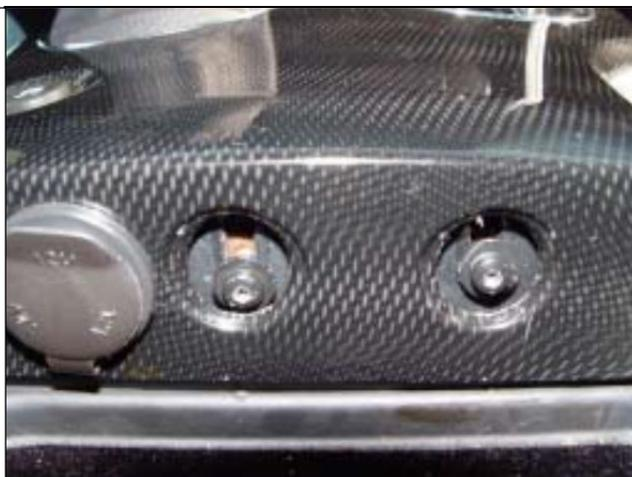
3. Pull up on sleeve around emergency brake uncovering bolts attaching center console.
