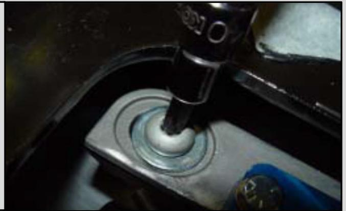
F. Remove the "L" pin from the pin hole and test the shifter through each gear.
