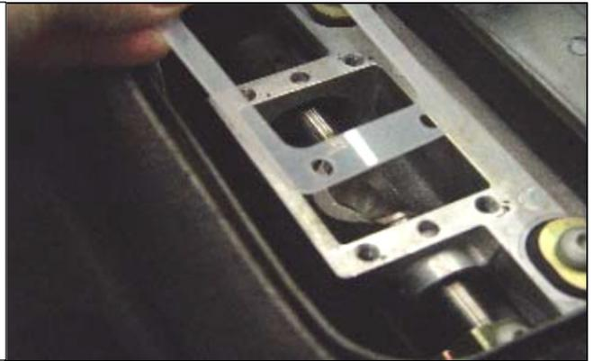
15. Install the B&M shifter. Secure the shifter to the transmission shifter base with the (4) provided 1/4" washers and 1/4"-20 screws. (Add a drop of medium-strength thread-locker (Permatex Blue or similar) to threads for added security.) Test shifter through all gears.
