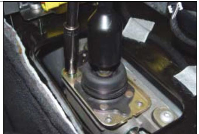
12. Gently remove the pivot cup from the bottom of the stick. For extra protection, use a towel between the channel locks.
