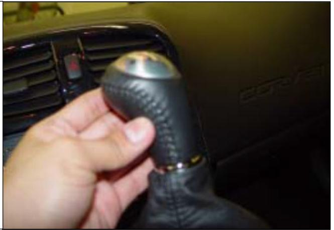
18. Reinstall the leather boot into the center console trim plate. Unclip the knob from the chrome collar and screw the provided bolt into the shifter, make sure the bolt presses firmly onto the knob. Clip the chrome collar back into the knob.
