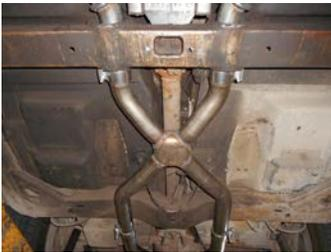
1b) Starting just behind cross-member, place provided 2.25" clamp onto expanded ends of X-pipe assembly **#86171S**, then slide it onto rear of manifold pipes (verifying connections are secure). Place stand under assembly rear and tighten clamps just enough allow for later adjustment.
