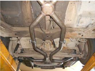
2) Place a provided clamp onto both outlets of X-pipe assembly **#86171S**. Place the expanded end of mid pipe **#86175S** onto the right outlet of the X-pipe assembly. Rotate the pipe up into position and support the rear of the pipe with a stand. Tighten the clamp enough to hold but still allow for adjustment. Repeat this step on the left side of the vehicle with pipe **#86176S**.
