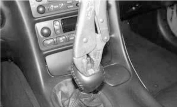
3. **Remove the T-shaped key from the knob.** (It may be pried up with 2 flat-tipped screwdrivers — one on each side of the key's T-shaped head — or pulled out with locking pliers.) Then unscrew the knob from the shift lever.
