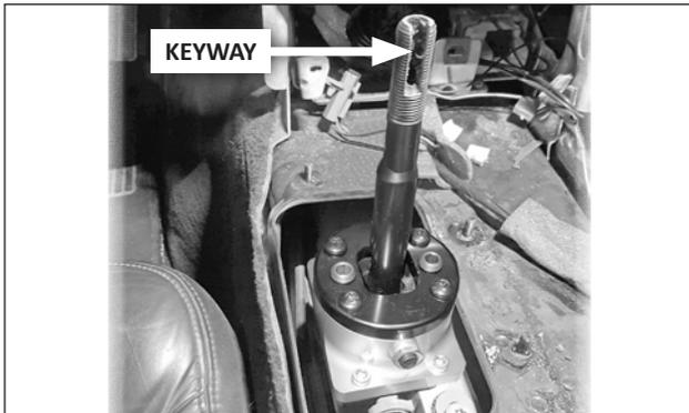
17. Orient the shifter with the shift lever keyway to the rear, and place it on the shift box, inserting the pivot cup into the shift linkage. Apply medium-strength thread locker to the 4 screws, and use them to secure the shifter to the shift box.
